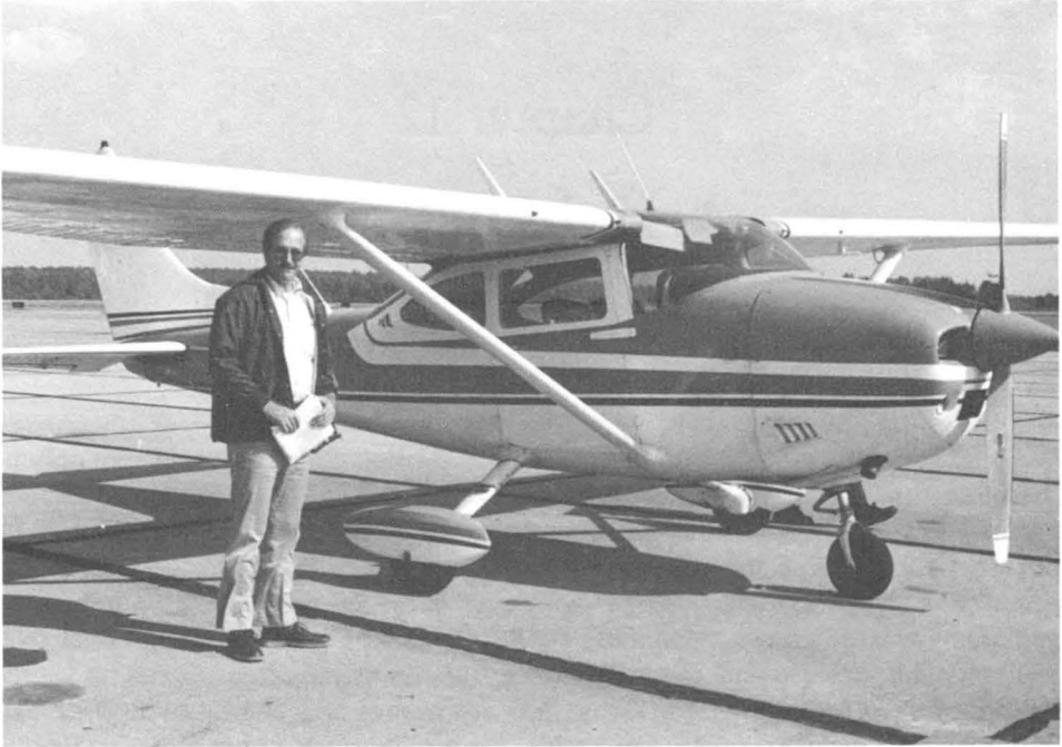
Figure 12.1 Photograph of a small fixed-wing aircraft used in an aerial survey of anglers. This airplane has its wing set above the fuselage, which permits relatively unobstructed views beneath the plane.
