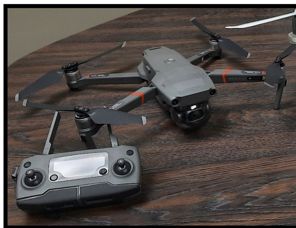
Figure 3 DJI Mavic 2 Enterprise Dual small unmanned aerial system (sUAS) platform used to conduct aquatic turtle surveys in the Sabine River Basin.
