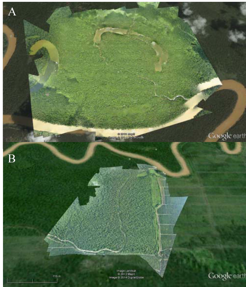
FIGURE 3. A) Stitched image of 280 ha flight flown at 0700 local time GMT+8, where the stitching quality was of high. B) Stitched image of 390 ha flight flown at 1400 local time GMT +8, where the stitching quality was of low.
