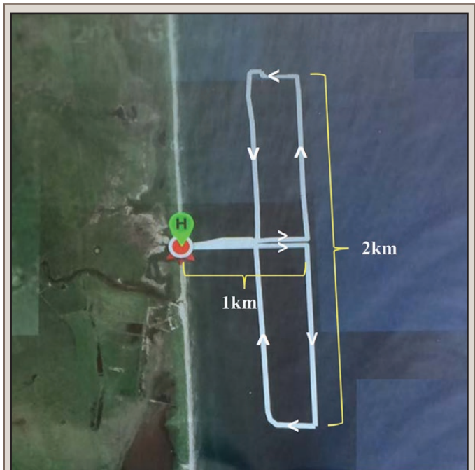
FIG. 3. Example of a typical survey using the UAV during the current study. Each location surveyed included 2 transects that were 2 km in length and parallel to shore. These transects were conducted at 0.5 and 1.0 km from shore. The operator's location is indicated by the "H". Two flights were required to complete the transects at each location, one to the north of the operator and one to the south of the operator as indicated by the arrows in the figure. These surveys were conducted at approximately 5-km intervals over a 30-km stretch of beach at Rancho Nuevo, Mexico.
