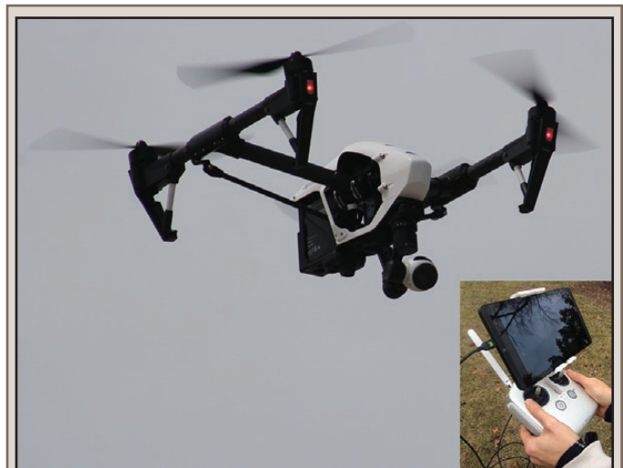
FIG. 1. In the current study, we used the DJI Inspire 1™ rotorcraft UAV platform for monitoring sea turtles in nearshore waters at Rancho Nuevo, Mexico. This UAV is equipped with a camera capable of up to 4K quality video. It provides a live, high-definition video feed up to 2 km from the operator. The controller interfaces with a tablet (NVIDIA Shield™ shown in the inset) running the DJI GO App™ to operate the aircraft.
