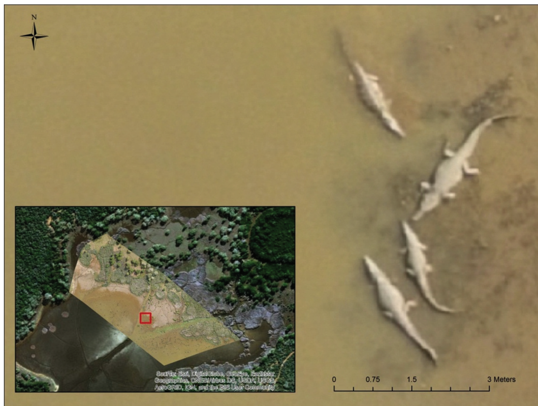
Fig. 2. Stitched image of 12 ha pilot flight flown at 55 m, where the produced 2D map quality is 2 cm/pix. The total length (TL) of the individual crocodiles observed were measured.
