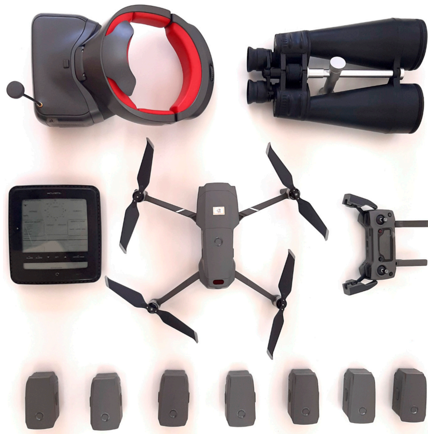
Figure 3. Main equipment used during field activities of the drone-monitoring in a natural environment: virtual reality mask—First Person View (FPV), Mavic 2 Zoom drone with extra batteries, long-range binoculars, and portable weather station.
