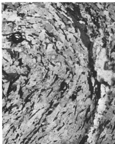
Figure 5. Magnification (X13) — Plane nicol: Microscopic fold in quartz-feldspar (zoned oligoclase, An_{17} ) — epidote-biotite-(chlorite) gneiss. The feldspars show a preferred orientation; the epidote is idioblastic. The fact that the flakes of biotite are practically not bent and that quartz shows no undulatory extinction indicates that dynamometamorphism took place before thermometamorphism (annealing process).
