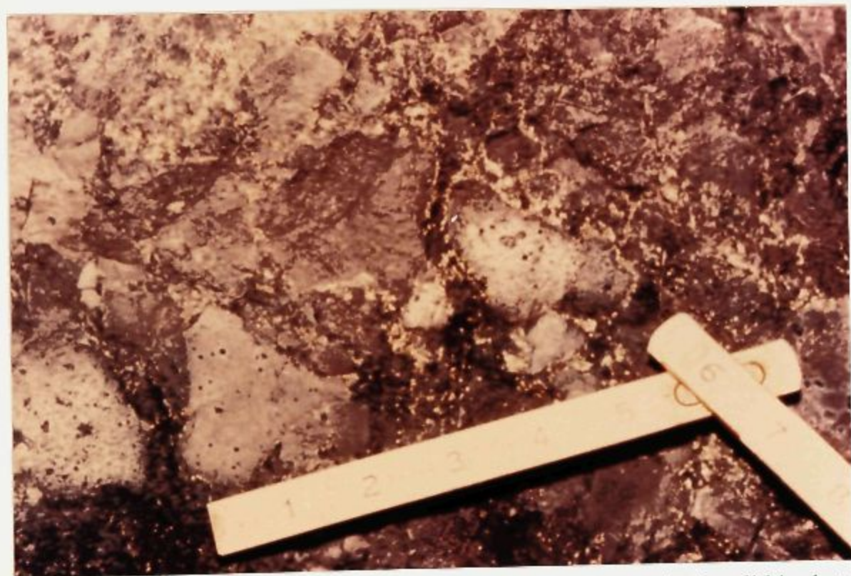
Plate C.4. Numerous sericitized andesitic "scoria" fragments and minor lithic clasts in a fine tuff matrix.
