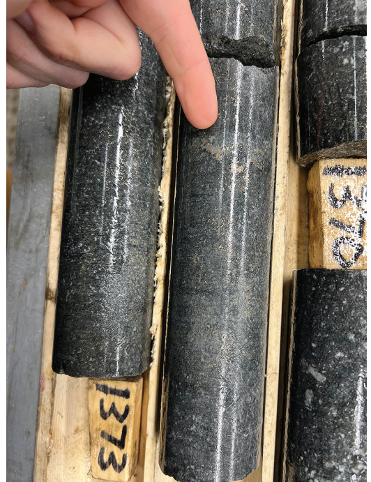
Geologist Dave Freedman [left] stands behind a row of core samples at KoBold's Cape Smith site in Nunavik, Que., Canada, taken from areas of interest to confirm AI predictions. Brownish flecks in the core sample above, KSC 22-07, reveal the presence of magmatic pyrrhotite.
