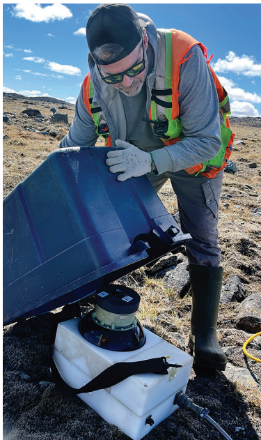
Audry Afango [far left] and Morgan McNeill work with a receiver on a ground electromagnetic loop in the middle of an angular boulder field in Nunavik, Que., Canada. On the right, McNeill, a geophysics technician, uses a superconducting quantum interference device (SQUID) to conduct a ground electromagnetic survey to pick up faint magnetic fields from conductive bodies underground.
