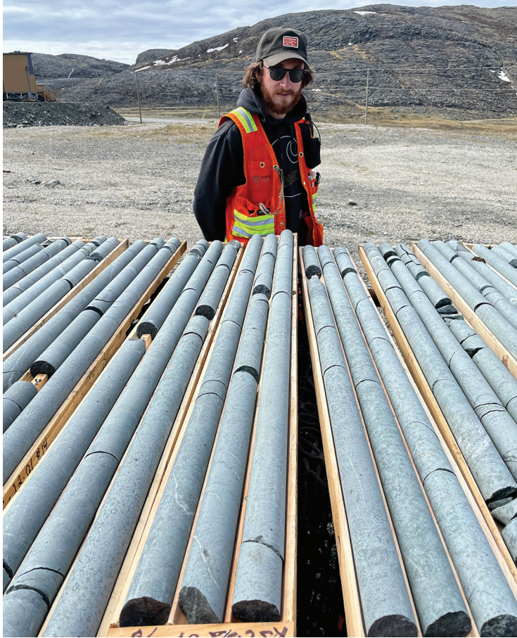
Geologist Dave Freedman [left] stands behind a row of core samples at KoBold's Cape Smith site in Nunavik, Que., Canada, taken from areas of interest to confirm AI predictions. Brownish flecks in the core sample above, KSC 22-07, reveal the presence of magmatic pyrrhotite.
