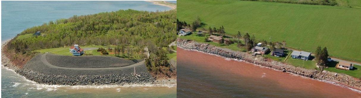
Figure A.4. Extreme example of residential coastal armouring near Melmerby Beach, Nova Scotia (left). Example of shoreline armouring near East Linden, Nova Scotia on Northumberland coast (right) (Nova Scotia Department of Natural Resources, 2011).
