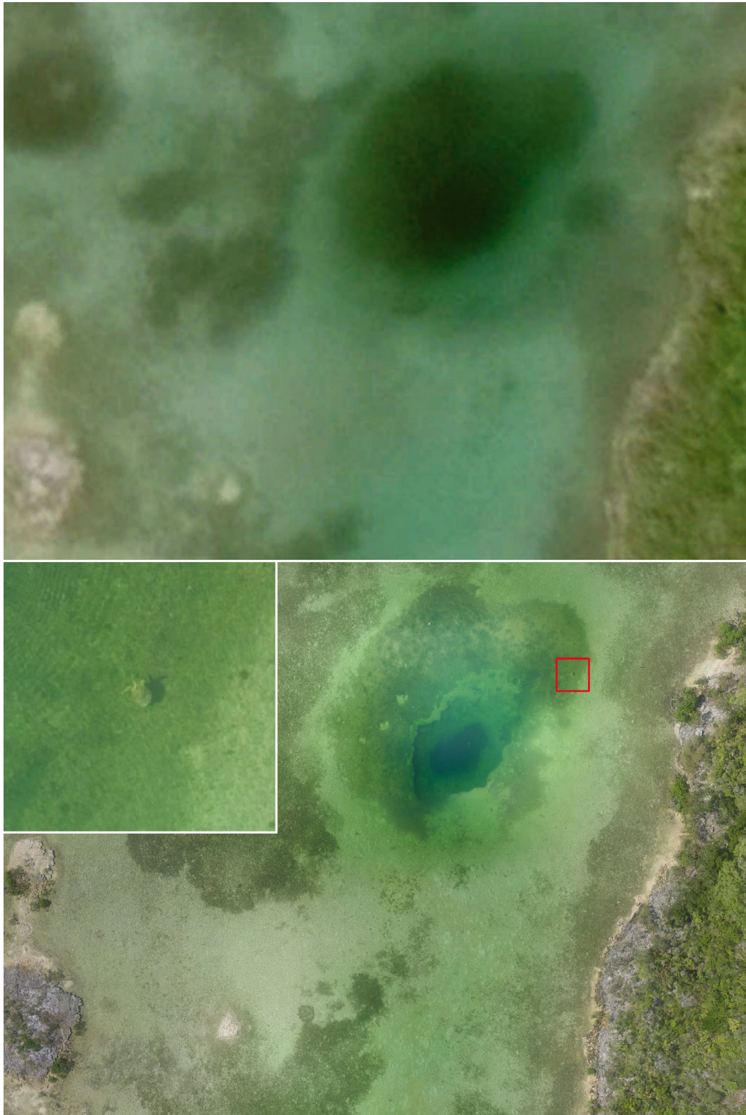
Fig. 5. Photogrammetric reconstruction of a section of tidal creek in the Bight of Old Robinson, Abaco, The Bahamas, with a 2 cm pixel resolution. Main images compare resolution between satellite (Google Earth; upper) and unmanned aerial vehicle (UAV; lower) derived imagery. Lower image inset displays the extreme detail that is readily possible using UAV data and photogrammetry (Image: E. R. Whitman, using a DJI Phantom 3 Advanced with a 2.7K HD camera at 30 m altitude)
