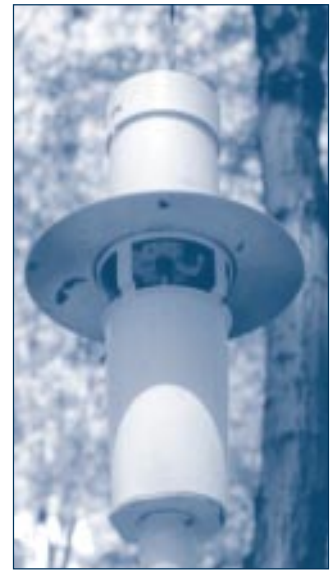
Luminoc®, a small light trap that can be suspended to catch all kinds of insects
