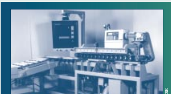
The colour grader for wood components, an innovation that makes better use of forest resources
